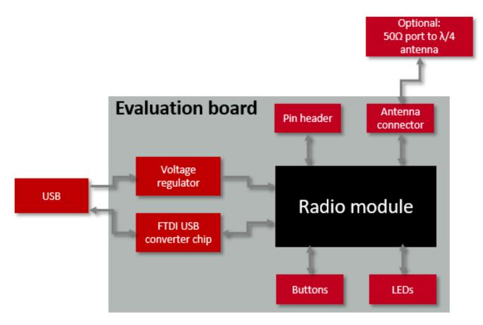
Figure 2: Block diagram
