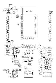
Figure 12: Assembly diagram
