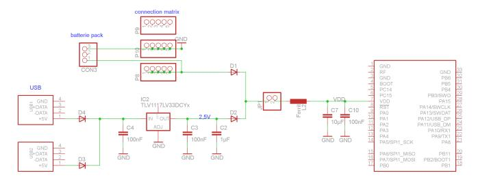
Figure 7: Power supply schematic
