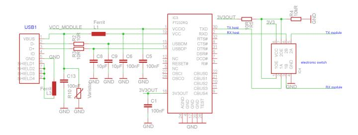
Figure 8: UART to USB converter: FT232R
